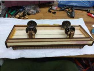
Glue the sole bar and axle box/wheel assemblies into place, ensuring that the wheels can rotate freely and there is not an excessive amount of end float.
