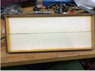
Mark the centre line of the floor. The distance between the sole-bars will be 75mm. Mark the position for the sole bars 37.5mm each side of the centre line, or thereabouts.
