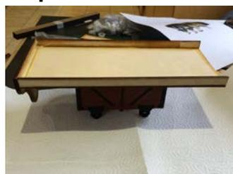
When dry glue each end on to the floor as shown.
