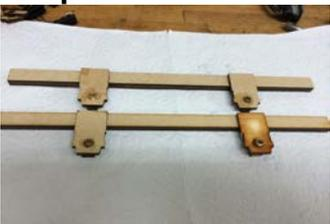
Fit the wheel bearings to the axle boxes. I use an epoxy resin adhesive.
