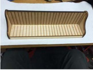
Glue the two back panels together, with the detail outwards. Glue between the ends as shown.
