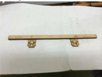
Glue the axle box assemblies, two per side. I glue them at 65mm from each end. If you glue them closer together, they will go around a tighter curve.
